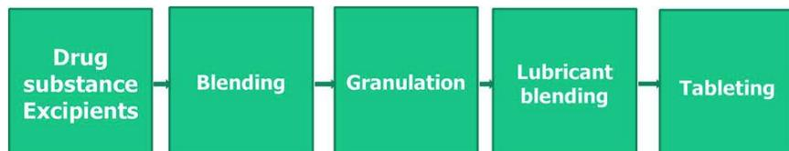
**Figure 1.** The tablet manufacturing process.
